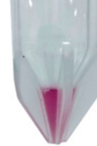
Figure 3: Example of 500 \mu L in the GELATION TUBE (DMEM is used for instruction purpose)
